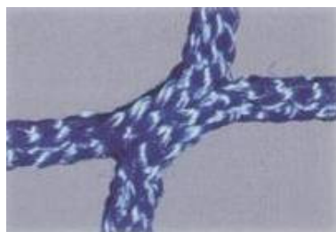
Figure 2: Raschel net does not contain knots
